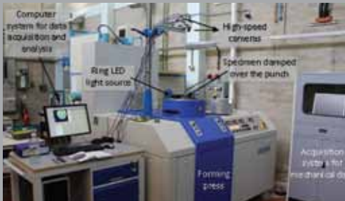
Figure 1. Materials Science Centre, The University of Manchester. Experimental setup including an acquisition computer system and a Hydraulic sheet forming press
